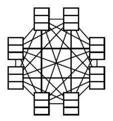
Sparse dependencies  $\Rightarrow$  exponentially fewer parameters; e.g., 20 state variables, three parents each DBN has  $20 \times 2^3 = 160$  parameters, HMM has  $2^{20} \times 2^{20} \approx 10^{12}$
