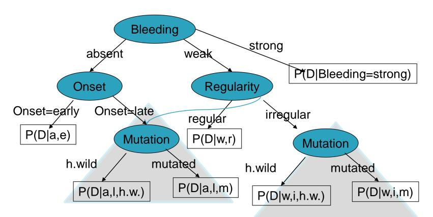
Decision tree: Each internal node represent a (univariate) test, the leafs contains the conditional probabilities given the values along the path.
