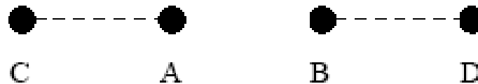
Fig. 2. Neighboring nodes A and B have different schedules. They synchronize with nodes C and D respectively.
