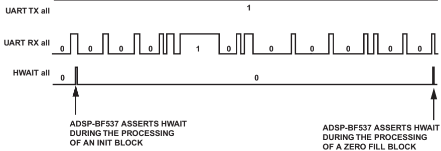
Figure 19-35. UART Init and Zero Fill Blocks
