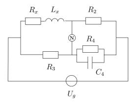
The so-called Maxwell–Wien bridge in the above figure measures the equivalent series model  $(L_x, R_x)$  of an inductance. The adjustable elements of the bridge are  $R_4$  and  $C_4$ , and  $R_2 = R_3 = 100 \Omega$ .
