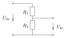
The figure displays a voltage divider made up of two resistors. The values of the resistors are  $R_1 = 49 \text{ k}\Omega$  and  $R_2 = 1 \text{ k}\Omega$ . The tolerance of both resistors is 100 ppm.
