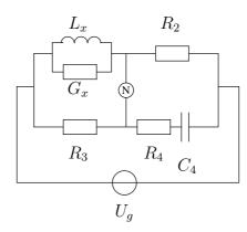
The so-called Hay-bridge in the above figure measures the equivalent parallel circuit model  $(L_x, G_x)$  of an inductance. The adjustable components are  $R_4$  and  $C_4$ , while  $R_2 = R_3 = 1 \text{ k}\Omega$ .
