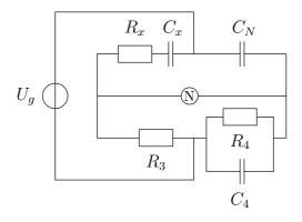
The so-called Schering bridge in the above figure measures the equivalent series model  $(C_x, R_x)$  of a capacitor. The adjustable elements are  $R_3$  and  $C_4$ , and  $R_4 = 10 \text{ k}\Omega$ ,  $C_N = 10 \text{ nF}$ .
