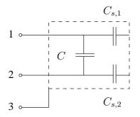
where C is the measured capacitor, while  $C_{s,1}$  and  $C_{s,2}$  are the stray capacitances.
