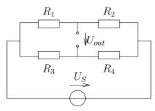
The output voltage of the bridge is the voltage difference between the two voltage dividers:
