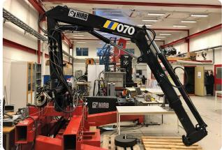
FIGURE 19 The tree-harvesting hydraulic crane.
