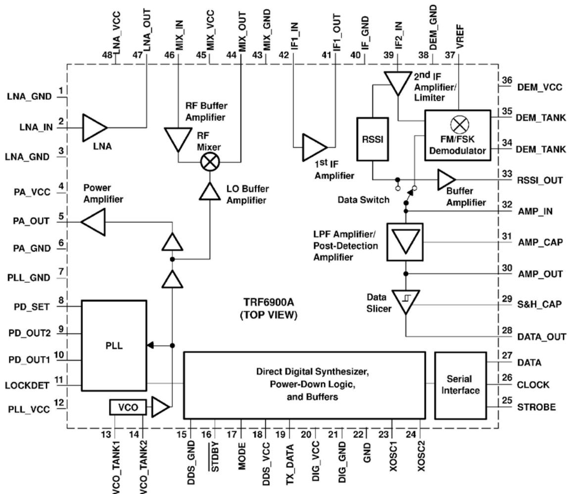
Fig. 10-1. Building blocks of the TRF6900A transceiver.
