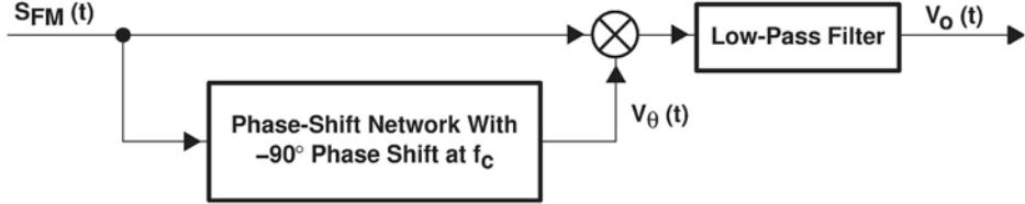
Fig. 10-5. The block diagram of frequency discriminator.
