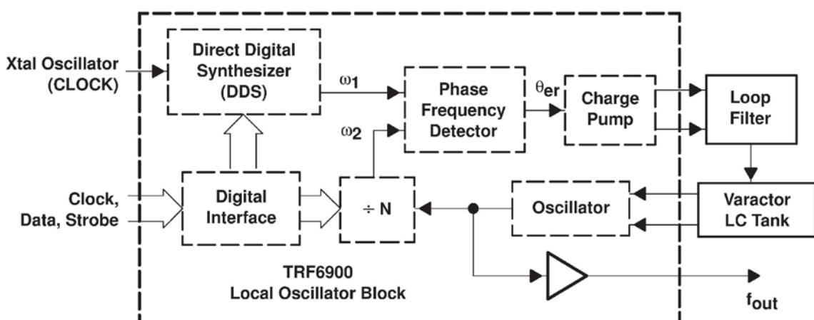
Fig. 10-3. Block diagram of the TRF6900A local oscillator.
