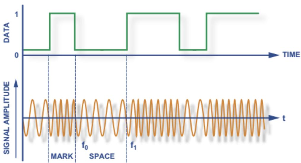
Figure 6. FSK modulation.
