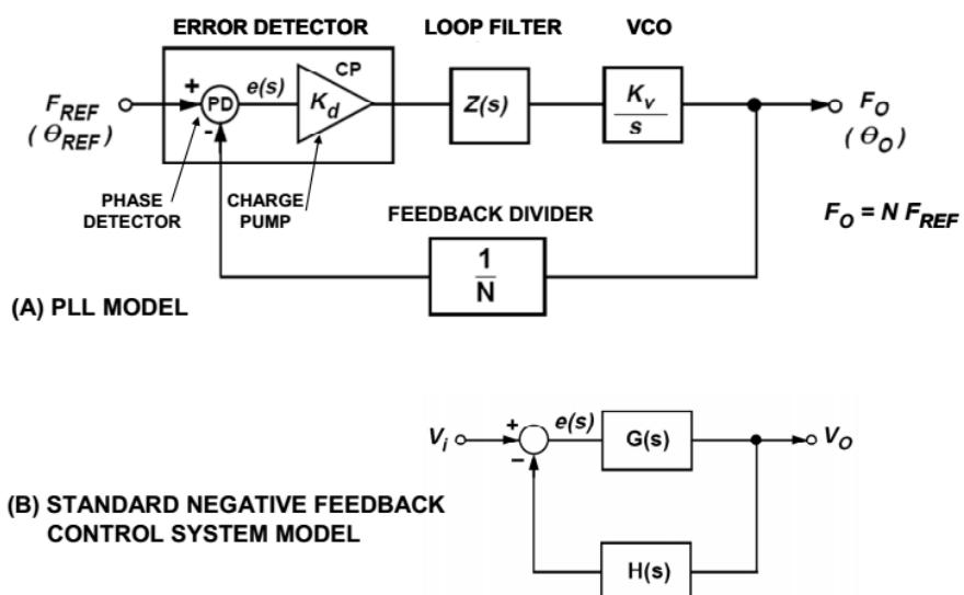
**Figure 1: Basic Phase Locked Loop (PLL) Model**
