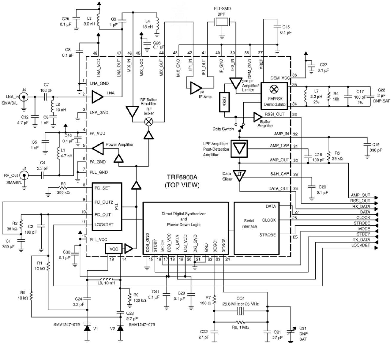
Fig. 10-2. Typical application schematics for the TRF6900A FSK transceiver. Note, one external IF channel (selection) filter is used, the IF frequency is 10.7 MHz.
