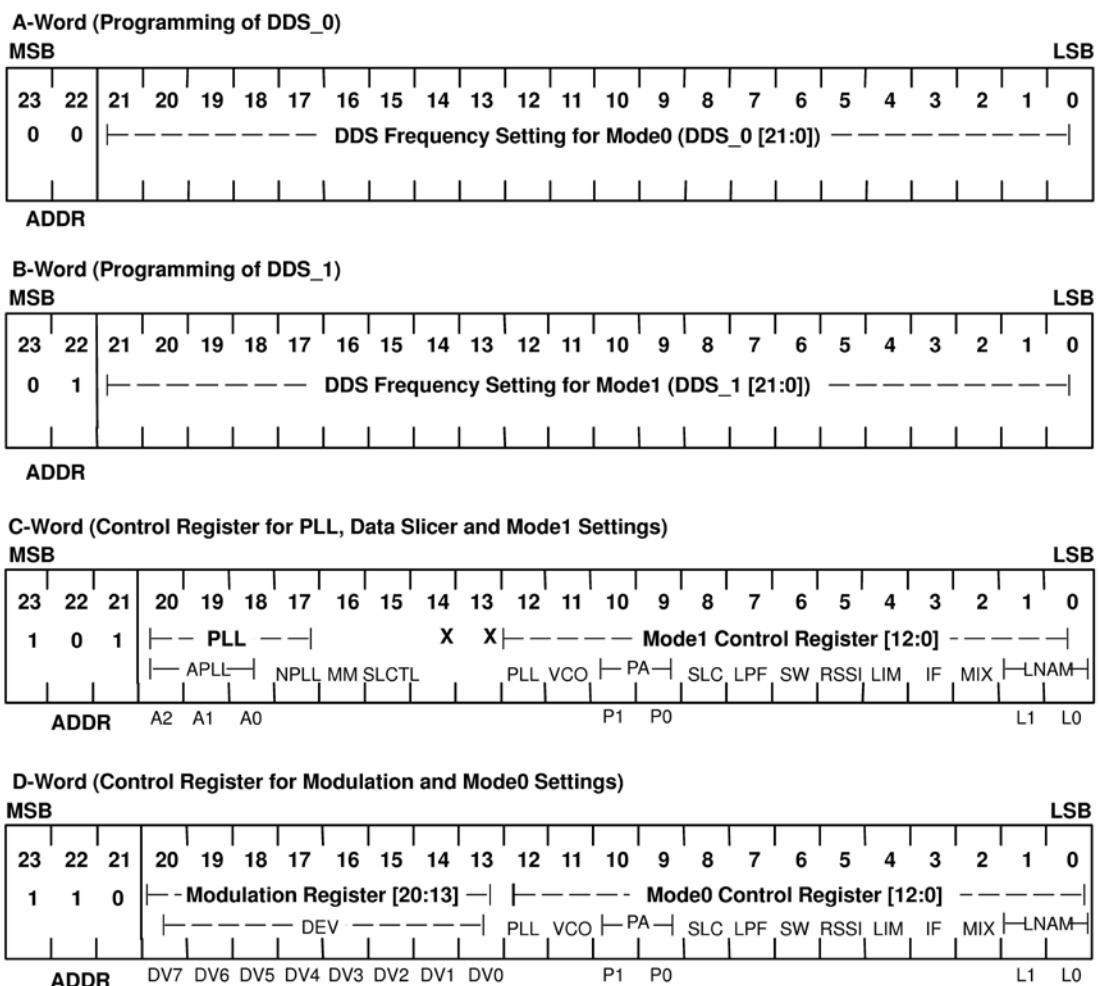
Fig. 10-6. Format of code words used to control TRF6900A integrated circuit.
