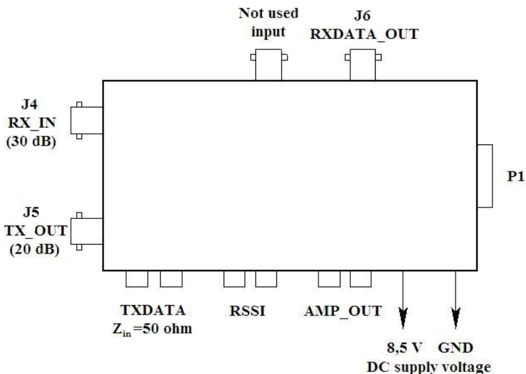
Fig. 10-11. Test set containing TRF6900EVM.
