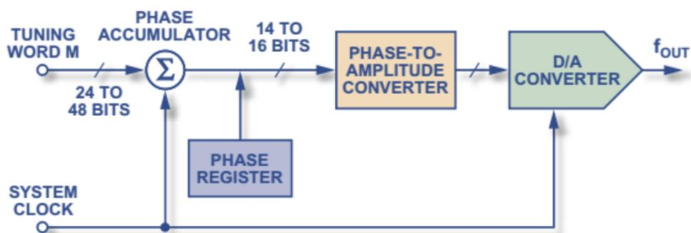
Figure 3. Components of a direct digital synthesizer.
