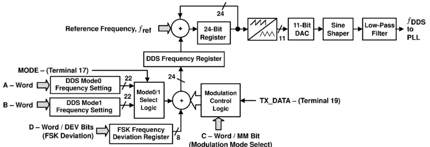
Fig. 10-4. Block diagram of the DDS used in TRF6900A.
