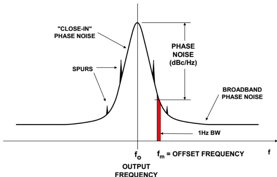
**Figure 5: Oscillator Phase Noise and Spurs**
