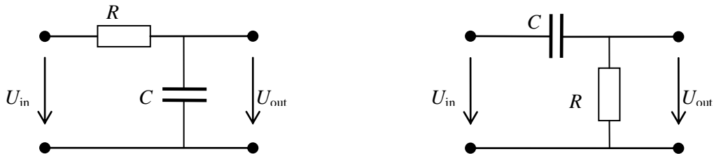
Figure 5-6. Schematic diagrams of first-order, low- and high-pass RC networks.
