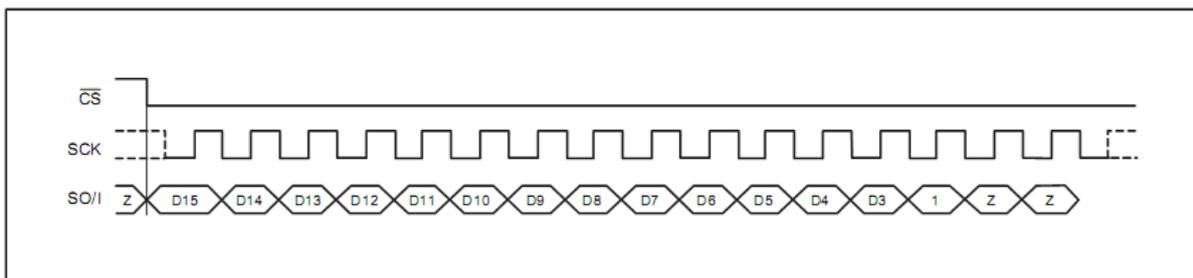
Transfer start is indicated by pulling the **Chip Select (CS)** low. Data is shifted out into wire **Serial Output (SO)** in the following 16 clock cycles (**SCK**). The 16 bit format is the one described above; the last 3 bits are don't care. The bits are shifted out on the **SCK falling-edge**.
