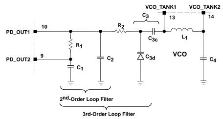
Figure 21. Basic 3<sup>rd</sup>-Order Loop Filter Structure
