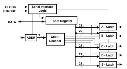
Figure 23. Serial Interface Block Diagram
