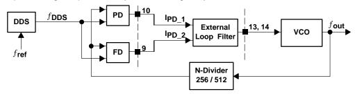
Figure 18. Basic PLL Structure
