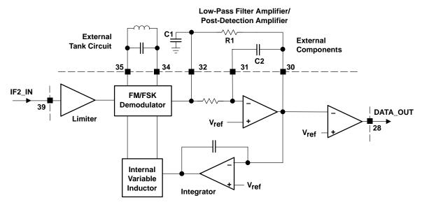
Figure 13. AFC Loop to Control the Data Slicer Decision Threshold
