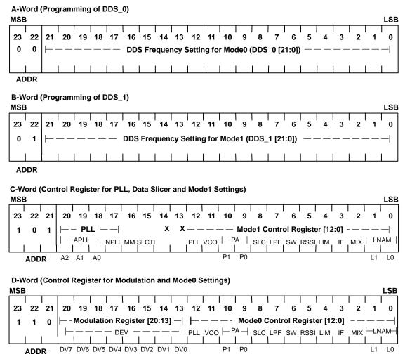
NOTE: Start programming with MSB and ensure that the CLOCK and DATA lines are low during the rising edge of the strobe signal.
