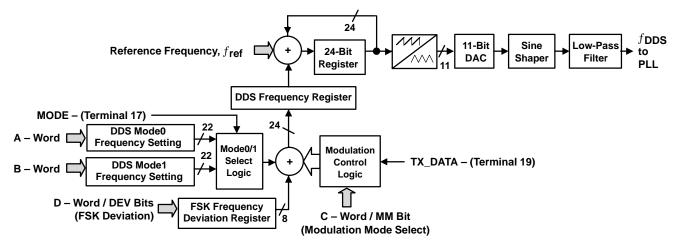
Figure 16. DDS Block Diagram as Implemented in the TRF6900A
