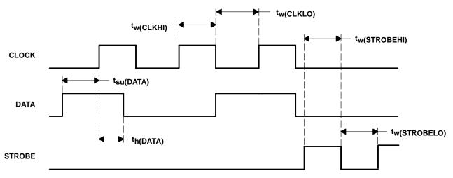
Figure 2. Serial Data Interface Timing
