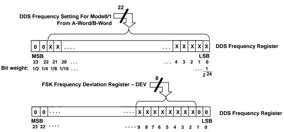
Figure 17. Implementation of the DDS Frequency and FSK Frequency Deviation in the DDS Frequency Register
