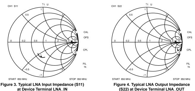
The low impedance of the LNA input can be easily matched to 50  $\Omega$  to interface with a filter or an RF switch. At the LNA open collector output, a filter network can be used for image suppression as well as impedance matching.
