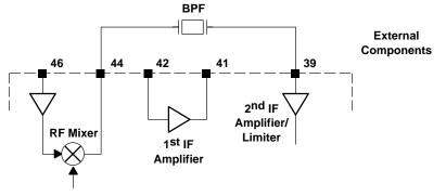
Figure 7. Bypassing the 1<sup>st</sup> IF Amplifier
