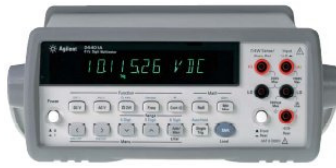
Digital multi-meter ( 6\frac{1}{2} digit) AGILENT 33401A
