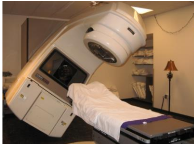
Between 1985 and 1987 the Therac-25 computer controlled radiation therapy system heavily overloaded 6 patients.
