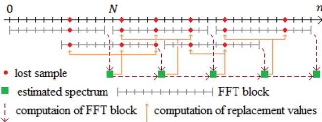
Fig. 4. Spectral estimation with replacement FFT method
