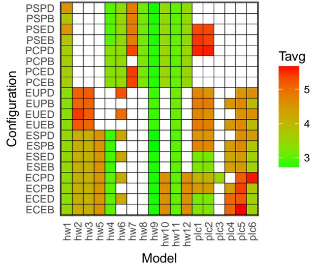
Fig. 3. Average execution time (milliseconds, logarithmic scale).
