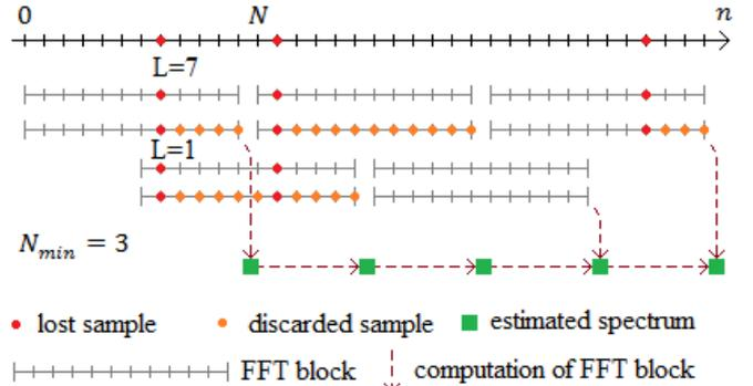
Fig. 3. Spectral estimation with zero padding FFT method
