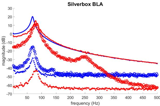
Fig. 2. The BLA of the Silverbox system for low (blue) and high (red) level of excitation. The FRF (full line), total distortion levels (circles) and noise distortion levels (dots) are shown. The size of the gap between the noise and total distortion level indicate how nonlinear the system behaves.
