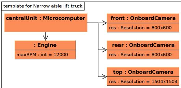
Fig. 7. Structure template of narrow-aisle lift truck
