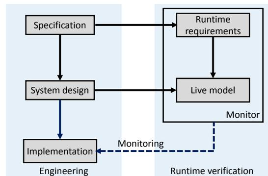
Fig. 1. Model-based runtime verification of a cyber-physical system.
