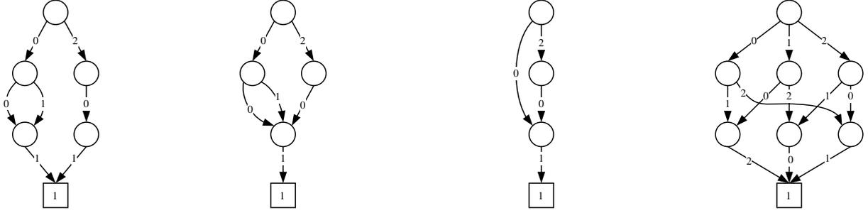
Fig. 1: An ordered MDD. Fig. 2: A quasi-reduced MDD. Fig. 3: A fully-reduced MDD. Fig. 4: MDD representation of  $\text{ALLDIFFERENT}(x_1, x_2, x_3)$ .
