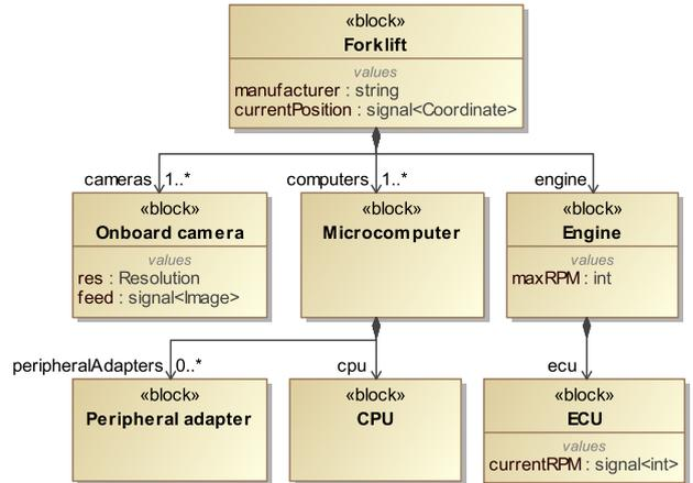
Fig. 2. Example metamodel with containment edges and attributes
