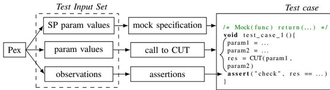
Fig. 1. Test case generation from Pex output
