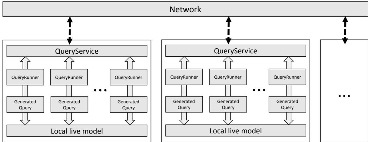
Fig. 7. Architecture of the distributed query evaluation.
