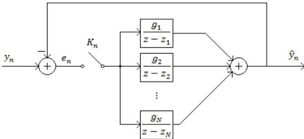
Fig. 2. Resonator-based observer for signals with lost samples.
