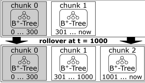
Fig. 2. The temporal rollover process by example
