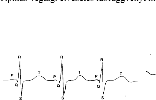
Fig. 1. Typical ECG waveform for three consecutive heartbeats. The analysis program's assignment is to locate each of the PQRST complexes correctly, and to measure the height, the width, and a multitude of other parameters as depicted in Fig. 2.
