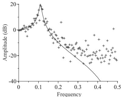
FIG. 1. Comparison of the true FRF  $G_0$  (—) with the estimated FRF  $\hat{G}$  (+)
