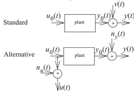
FIG. 4. : Standard and alternative noise assumption.
