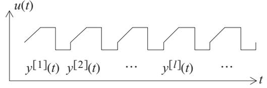
FIG. 3. Processing periodic excitations:  $y^{[l]}(t)$  is the  $l^{\text{th}}$  period.
