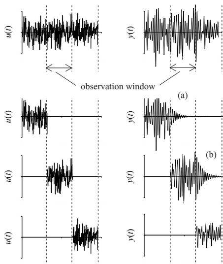
FIG. 2. : Illustration of the effect of the finite observation window.
