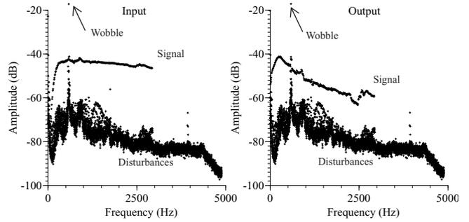
FIG. 7. Pilot test with a special odd multisine signal.
