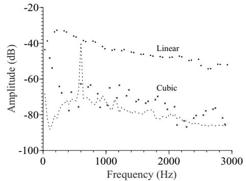
FIG. 9. nonlinearity test: power on the FRF measurement frequencies (linear), detected distortions after compensation for the linear feed through (cubic), ---  $\sigma_Y$ .
