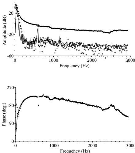
FIG. 10. : Comparison of the estimated transfer function (full line) with the measured FRF (dots). The residuals (+) are compared to the 95% noise level (thin full line).
