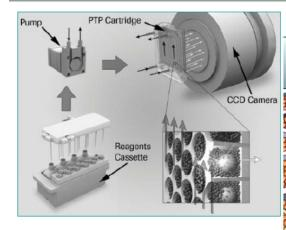
• A nucleotide-incorporation event in containing well template  $\rightarrow$ a pyrophosphate release > picotiterplate well–localized luminescence  $\rightarrow$ transmitted through the fiber-optic plate -> charge-coupled device camera
