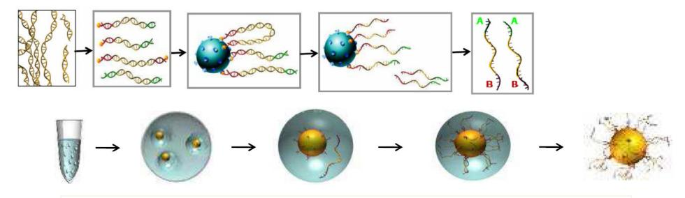
• PCR that occurs within **aqueous microdroplets** separated by oil (up to 1000 of independent reactions /ul)
