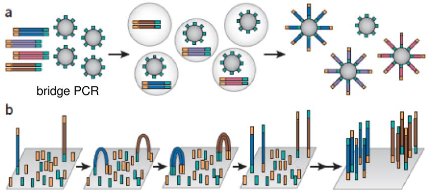
The immobilization of spatially separated template sites allows thousands to billions of sequencing reactions to be performed simultaneously.
