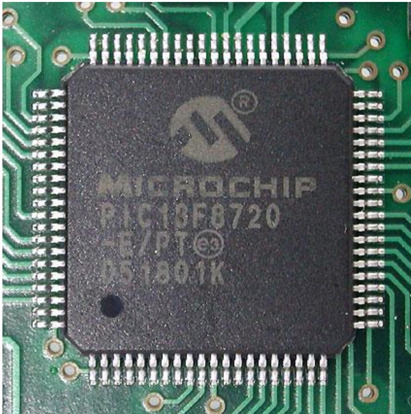
PIC 18F8720 microcontroller in an 80-pin TQFP package (12 x 12 x 1mm)
