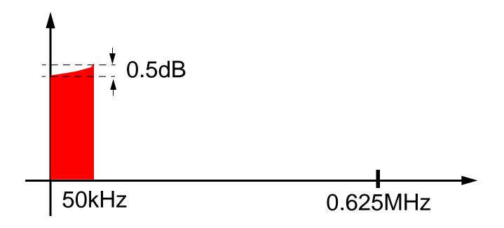
....therefore the decision of this final stage filter must be done very carefully to correct for the droop.
