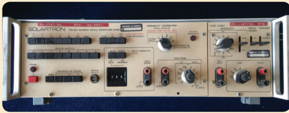
FIGURE S2 A pseudorandom binary signal generator from the 1960s used as an example in laboratories at the School of Engineering, University of Warwick. Dedicated generators to generate maximum length binary sequence and related signals like the inverse repeat binary sequence were built and commercialized. Besides the original signal u(t) , a copy with a user adjustable delay u(t - \tau) was also generated. This allowed the correlation y(t)u(t - \tau) to be measured using analog correlators, making a direct measurement of the impulse response g(\tau) possible.
