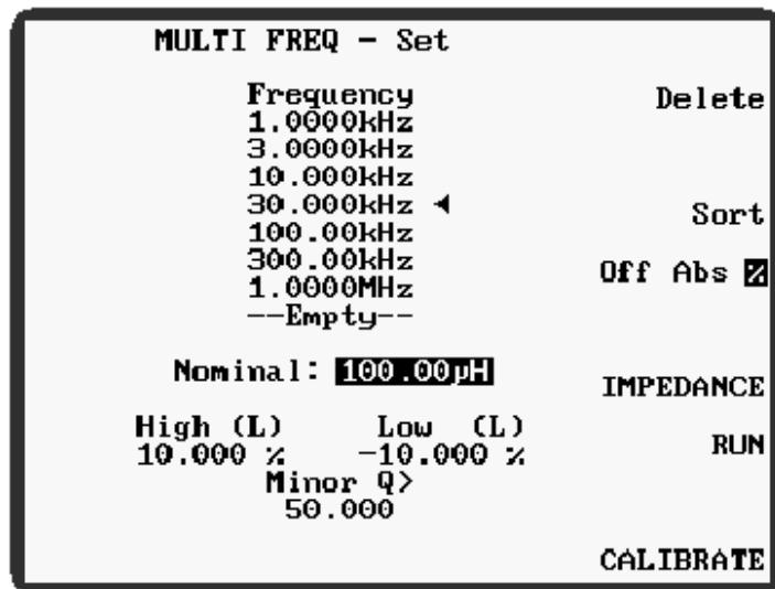
Figure 5-41 MULTI FREQ – Set Display Example
