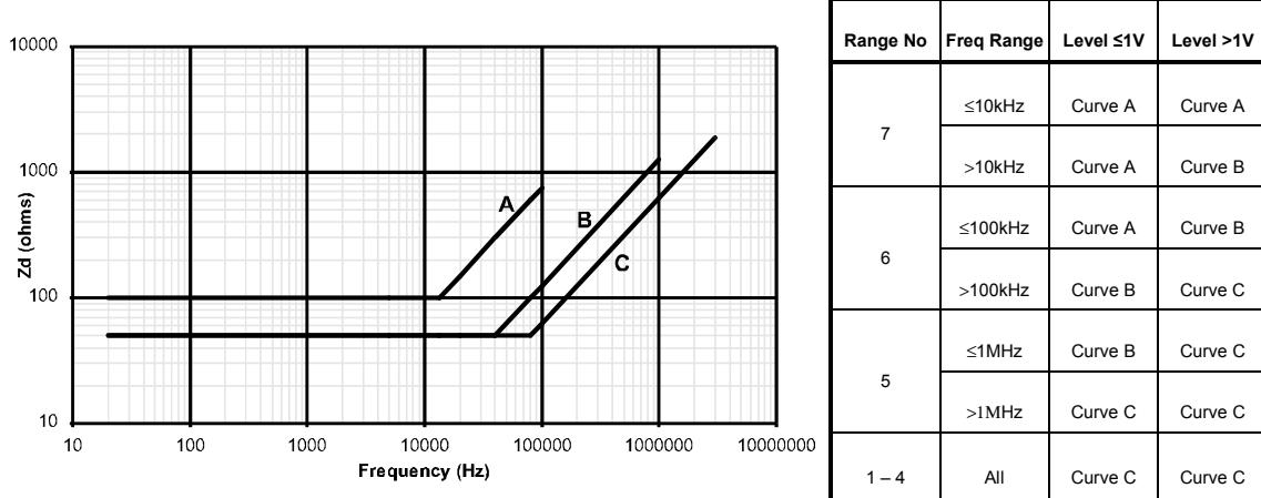
Figure 5-5 Effect of shunt loading on current terminal
