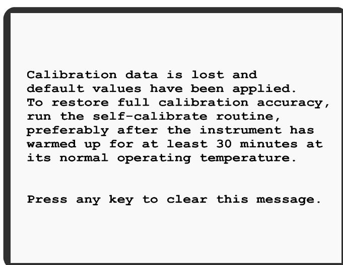
Figure 4-25 Calibration Data Lost
