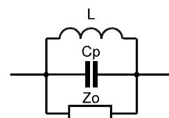
Figure 5-48 Parallel Equivalent Circuit
