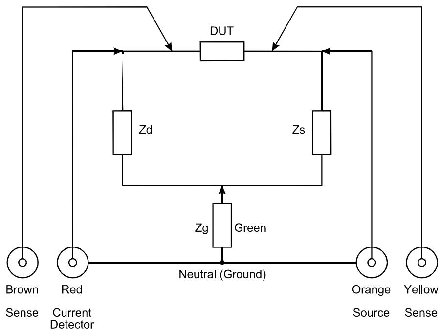
Figure 5-4 In-Circuit Measurements
