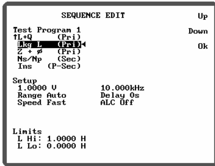
Figure 5-33 SEQUENCE EDIT MODE:Moving a Test Step
