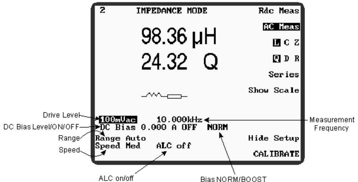
Figure 4-34 Non-Soft Key IMPEDANCE MODE Parameters
