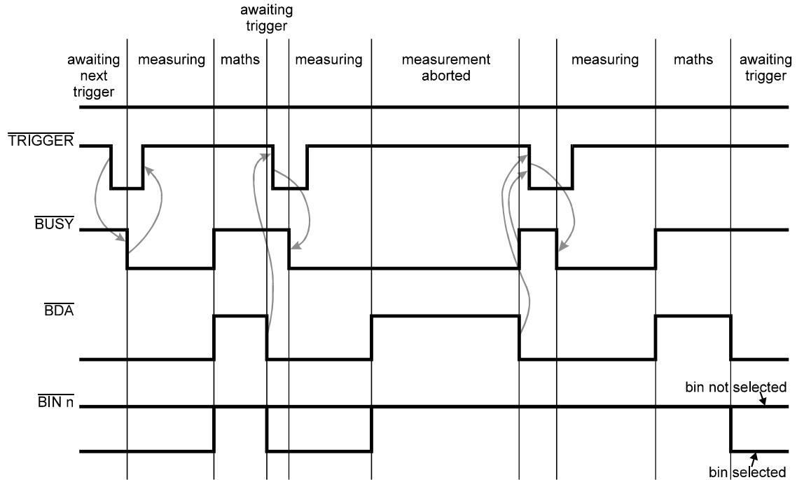
Figure 4-3 Standard Bin Handler Timing
