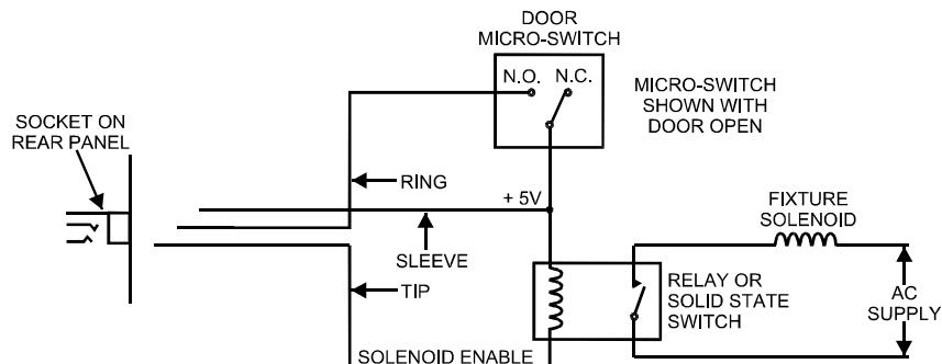
Figure 4-2 Typical Bias Interlock Fixture
