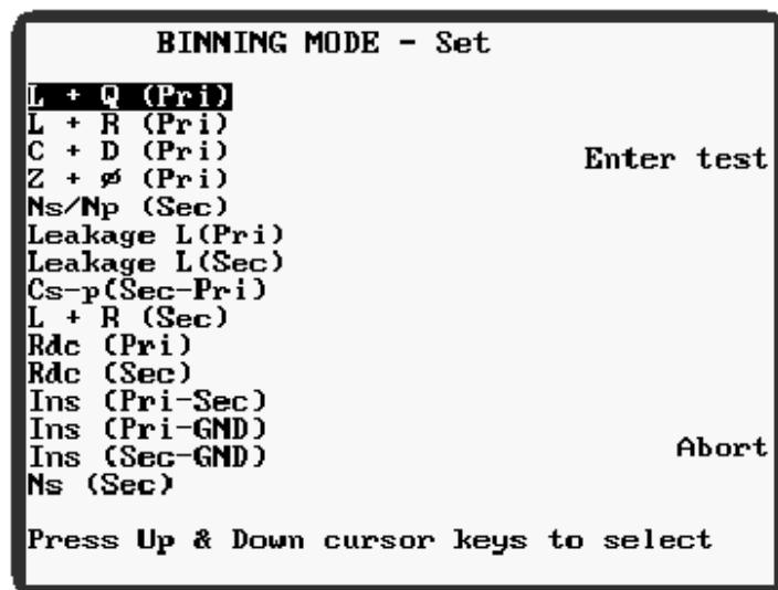
Figure 5-21 BINNING MODE – Set, Measurement Options
