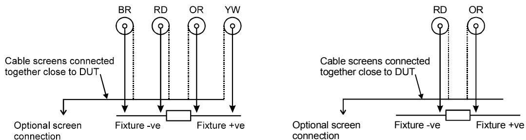
The four cables should be laced together with RED and BROWN diagonally opposite within the harness as shown below
