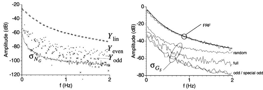
Fig. 5. Hair dryer experiment. Left side: detection of nonlinear distortions. Right side: impact of the excitation signal on the uncertainty ( $\sigma_{G_s}$ ) due to stochastic nonlinear distortions.
