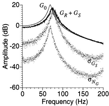
Fig. 1. Measurement of the related dynamic system ( $G_R$ ), the underlying linear system, the stochastic nonlinearities ( $\sigma_{G_S}$ ), and the noise level ( $\sigma_{N_G}$ ).
