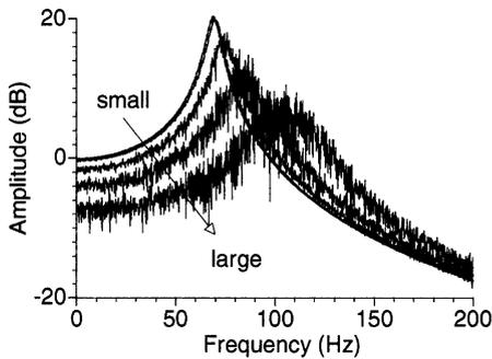
Fig. 2. Evolution of the related dynamic system for growing excitation levels: 34, 54, 127, 253, and 507 mV<sub>RMS</sub>.
