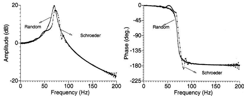
Fig. 6. Impact of the phase of the multisine on the measured FRF (RMS value of 54 mV). Random: odd random multisine with 1342 components. Schroeder: odd multisine with Schroeder phase. This signal acts like a swept sine.
