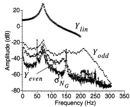
Fig. 3. Detection of nonlinear distortions at the output of the nonlinear circuit using an odd–odd multisine. x: linear + odd nonlinear contributions; +: even nonlinear contributions; •: odd nonlinear contributions.
