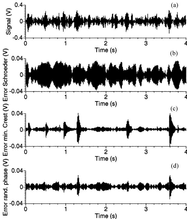
Fig. 7. Simulation error for the linear model obtained, respectively, with a Schroeder (b), random phase minimal crest factor multisine, (c) and random phase multisine (d), (a) shows the output signal of the circuit when driven with a normally distributed noise excitation.
