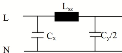
Fig. 8. Symmetric model of the network filter
