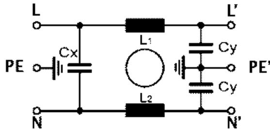
Fig. 7. The schematic of the network filter
