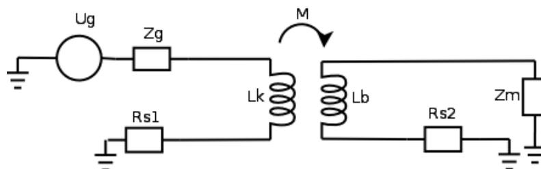
Fig. 2. Substitution of the inductive coupling for the measurement
