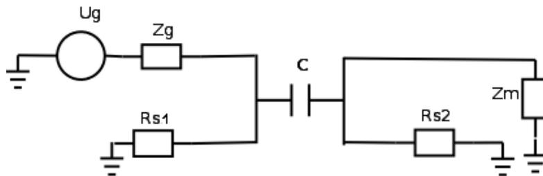
Fig. 4. The measurement substitution of the capacitive coupling
