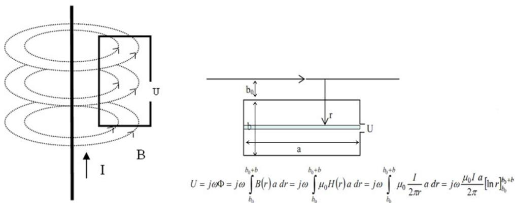
Fig. 1. Model of the inductive coupling
