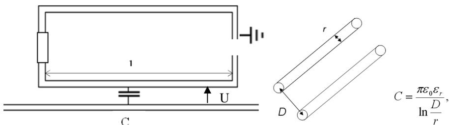
Fig. 3. Model of the capacitive coupling
