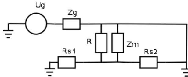
Fig. 6. The measurement substitution of the galvanic coupling
