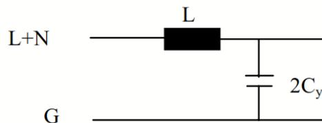
Fig. 9. Asymmetric model of the network filter
