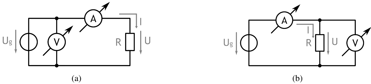
Figure 1: Measuring power with voltage and current meter
