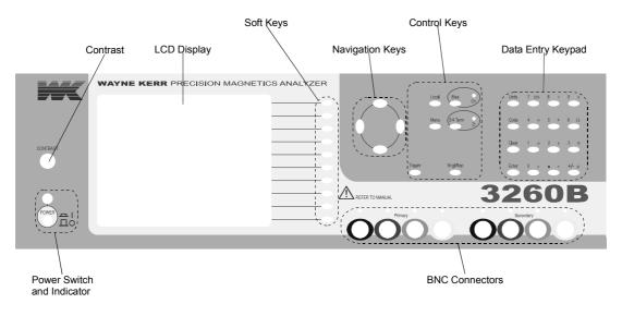
Figure 4-4 The 3260B Front Panel
