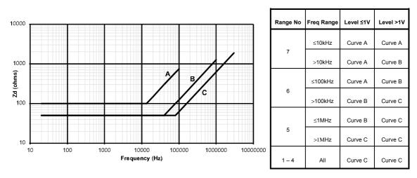
Figure 5-5 Effect of shunt loading on current terminal
