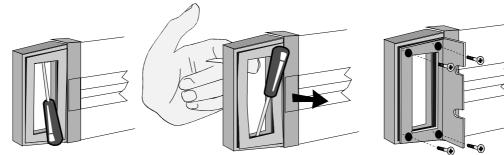
Insert small screwdriver into the gap between insert and handle body. Prise away one end slightly and hold in position with finger. Note operation of insert with styling cut-out opposite cut-out in handle.
