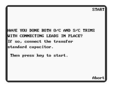
Figure 4-31 HF Lead Compensation
