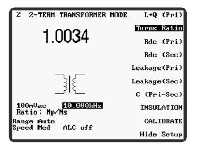
Figure 5-6 Example of Measuring Turns Ratio in TRANSFORMER MODE
