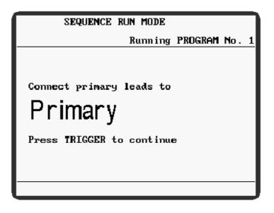
Figure 5-34 SEQUENCE RUN MODE: Connection Prompt
