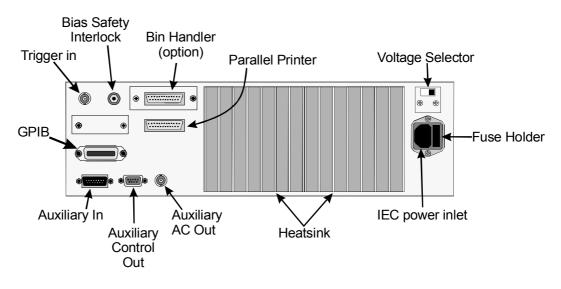
Figure 4-1 The 3260B Rear Panel
