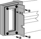
Insert rack mounting bracket into recess in handle in attitude shown and secure firmly with 4 M4x10 C'SK HD screws supplied.
