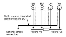
The four cables should be laced together with RED and BROWN diagonally opposite within the harness as shown below
