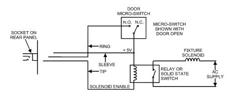
Figure 4-2 Typical Bias Interlock Fixture
