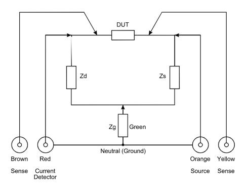
Figure 5-4 In-Circuit Measurements
