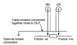
Figure 3-3 2 Terminal Measurement
