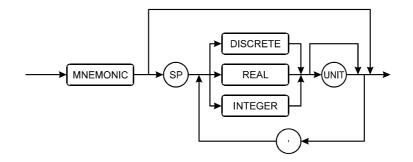
Figure 6-2 GPIB Command Structure
