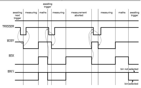
Figure 4-3 Standard Bin Handler Timing
