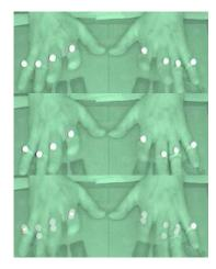
Figure 1.10. The odd field (top), even field (middle) and the two fields displayed as one frame (bottom) recorded with the PAM during finger-tapping.
