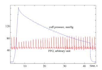
Figure 6.19. Time functions of cuff pressure and PPG signal during measurement. Loosely wrapped up cuff, pulses in PPG signal do not disappear.
