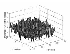
Figure 1.14. Noise of a CCD sensor: the difference of two images taken from the same scene.
