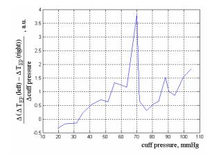
Figure 6.18. The rate of increase in  $\Delta T_{EP}$  as cuff pressure increases during slow inflation. Maximum increase is when cuff pressure equals diastolic pressure.
