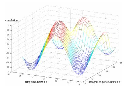
Figure 6.10. Correlation between  $\Delta T_{EP}$  and the integral of air flow over a time interval. Length of integration period and delay of pulse wave arrival at the fingertip to this interval are varied to find maximal correlation.
