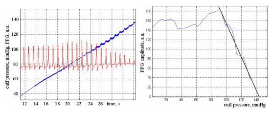
Figure 6.16. Amplitude of pulses in PPG signal as cuff pressure slowly increases.
