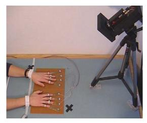
Figure 1.12. The measurement set-up for the tapping-test.
