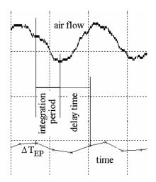
Figure 6.9. Definition of delay time and integration period for the compensation of the modulation in  $\Delta T_{EP}$  caused by breathing.
